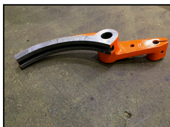
Bar feed adjustment lever Ref : 91858 SAS16
