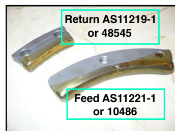
Feed and Return Pads Ref : 10486(feed) 48545(return) AS14
