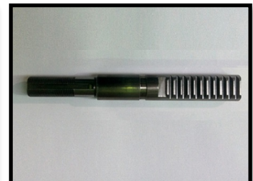
Rack station 1, 2, 3 & 4 Ref : 97719 BS20
