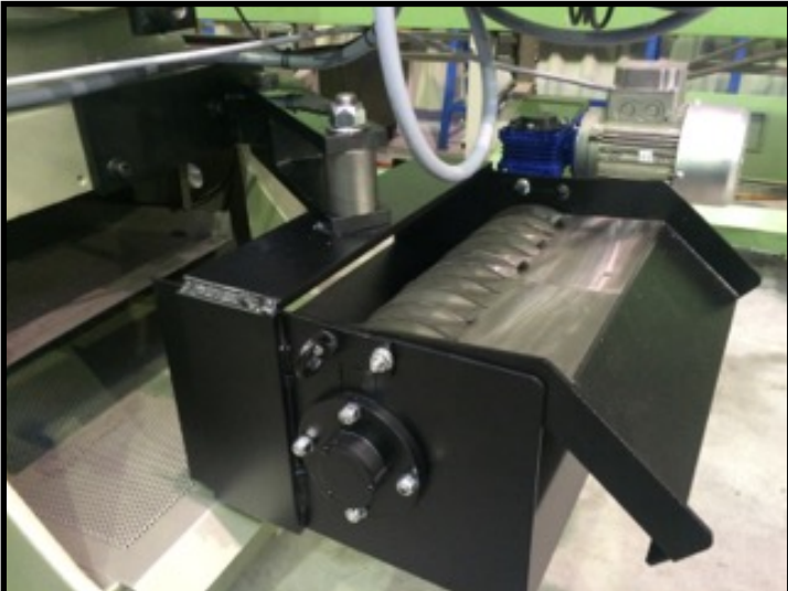
ARTICULATED MAGNETIC CONVEYORS SAMO AS14 - SAS16 - SAS16.6
