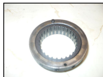
Adjustment ring of clutch Ref : 202009 AS14 - SAS16
