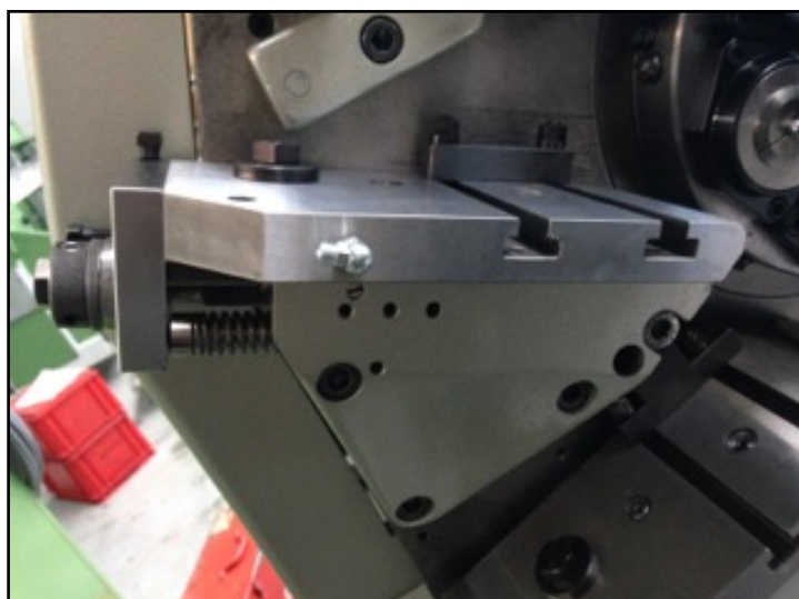
Slide station 1 Ref : 108677 AS14 - SAS16 - SAS16.6
