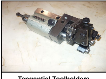
Tangentiel Toolholders Station 1 to 5 Ref : 104628 - AS30/10 AS14 - SAS16 - SAS16.6
