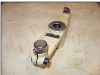
Non stop sub spindle feed lever Ref : AS28/7 AS14 - SAS16 - SAS16.6
