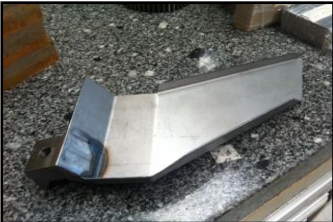
CHUTE EVACUATION FOR PIECE
